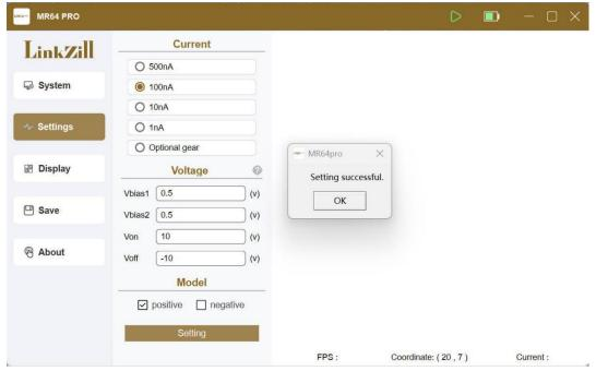
b. Click the green triangle icon at the top-right corner to start acquisition. The current frame rate, coordinates, and current value of the selected point will be displayed below the imaging area. During operation, the icon changes to a red rectangle. Click it again to stop sampling. Access the "Display" menu (See figure below) to adjust the image: The top three buttons perform 90° clockwise rotation, left-right flip, and top-bottom
