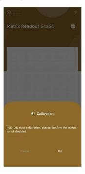
②. 0 grey level calibration: Make sure the TFT array is fully shielded to minimize the photocurrent. Click the "OK" button to set the 0 grey level (shown in the following image).
