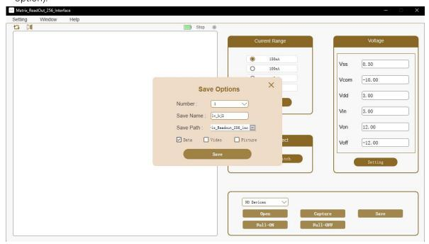
**Full-ON:** Perform independent 255 grayscale calibration for each pixel. After ensuring that the array sensor is in an unobstructed state, click the "Full-ON" button to record the current at this moment, corresponding to the 255 grayscale signal (white).
